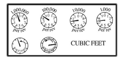
To take your reading, read the row of four dials in order from left to right. Note that some dials rotate clockwise while others operate counterclockwise. Beginning with the dial on the far left, record the number which each dial hand has just passed. The reading in our illustration is 0-8-2-7. To determine how much natural gas has been used since the previous reading simply subtract the previous reading from the current one.
